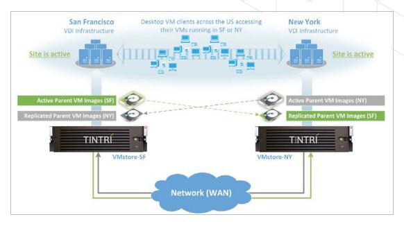
Figure 16: VDI high availability example, spanning two data center locations
