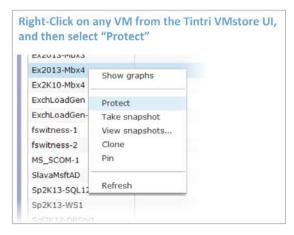
Figure 13: Setting per-VM snapshot protection and retention schedules
