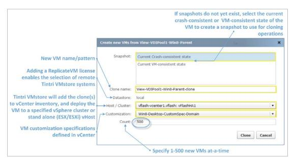
Figure 15: Per-VM cloning using the Tintri VMstore UI
